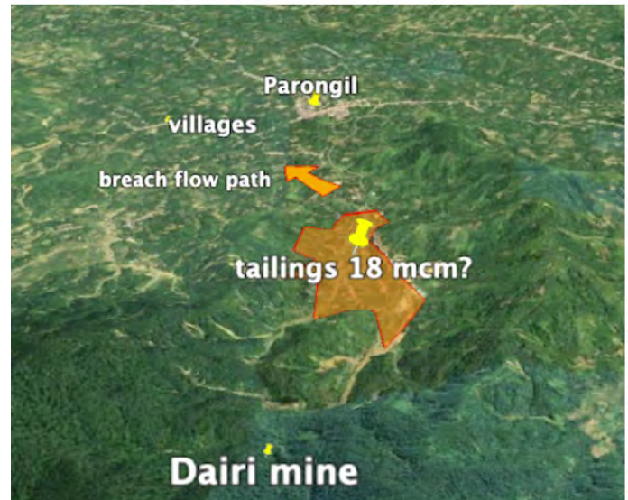
Figure 4. Path of mud wave if a breach occurs.
